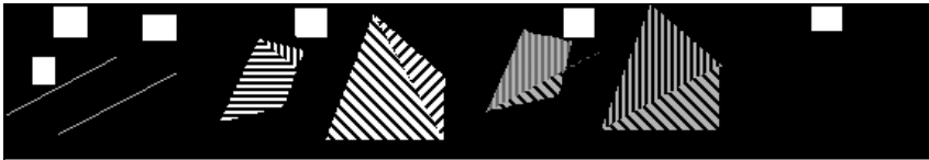
Figure 1. The first layer, P_1 , for scene (a) is made up of parts of nearest facing polygons (b). The second layer, P_2 is made up of parts of back facing polygons (c). The intersection of these two layers in image space creates silhouette edges (d).
